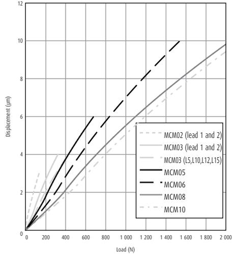
Fig. 4.2 MCM Series rigidity in radial direction
