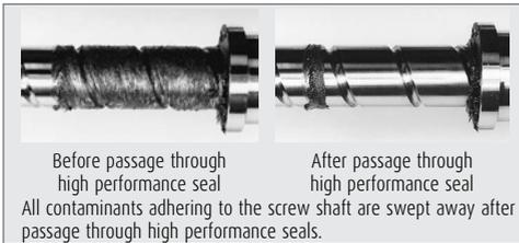
Fig. 2 Contamination before and after particle penetration test
