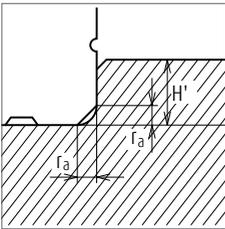
Fig. 6 Shoulder for the rail datum surface
