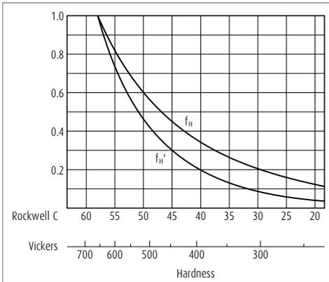
Fig. 2.6 Hardness coefficient
