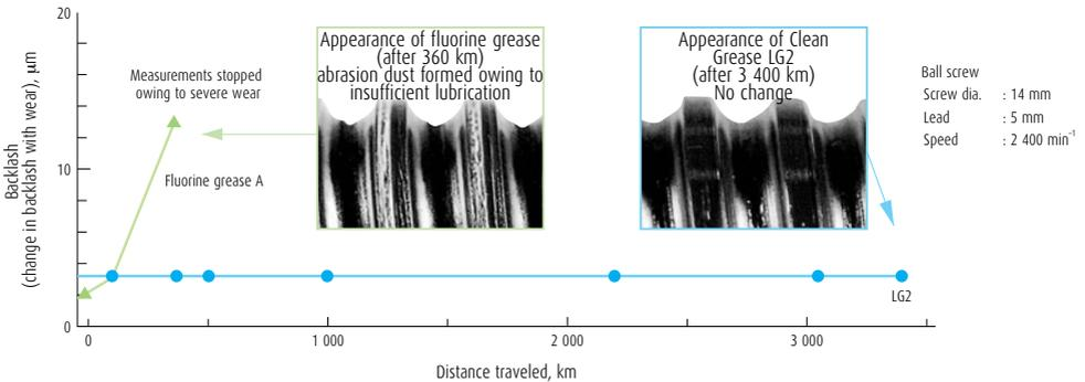
Fig. 4.6 Results of ball screw durability test
