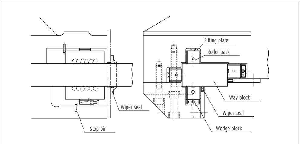
Fig. 7 Design of the roller pack pocket (example)
