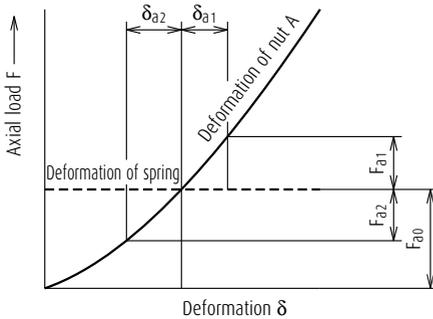
Fig. 6.5 Deformation curve of constant pressure preloaded nut
