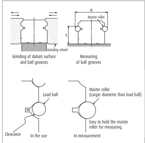
Fig. 4 Processing and measuring grooves
