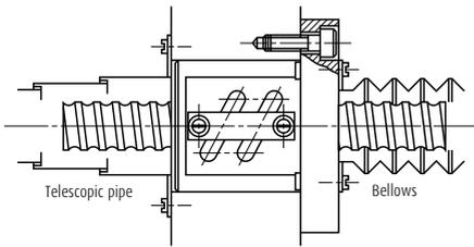
Fig. 10.1 Dust prevention by telescopic pipe and bellows
