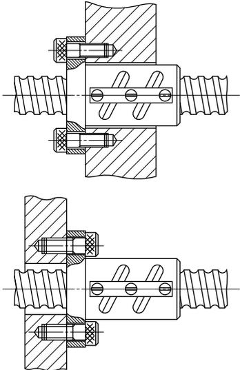
Fig. 15.5 Fixing a ball nut by flange
