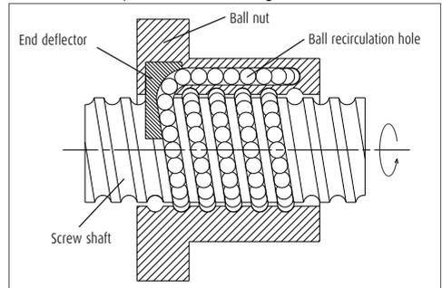
Fig. 4 Structure of end deflector recirculation system
