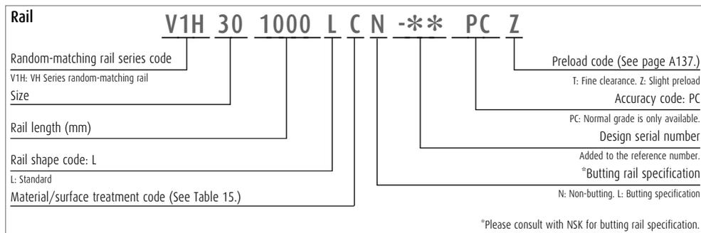
The reference number coding for the assembly of random-matching type is the same as that of preloaded assembly. However, the preload code of "fine clearance T" and "slight preload Z" is only applicable (refer to page A137).
