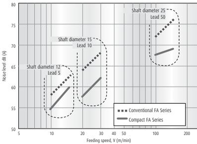
(Microphone was positioned at a distance of 400 mm for all noise levels)
