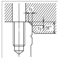
Fig. 9 Shoulder for the ball slide datum surface
