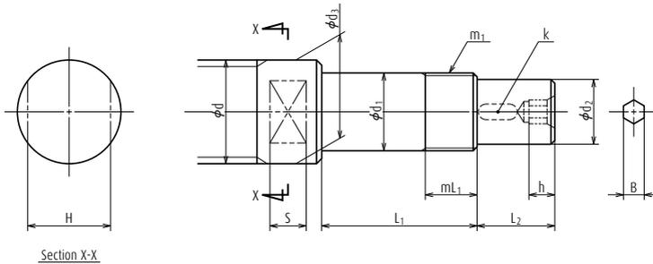
Fig. 4.4 Configuration of standard shaft end (drive side)
