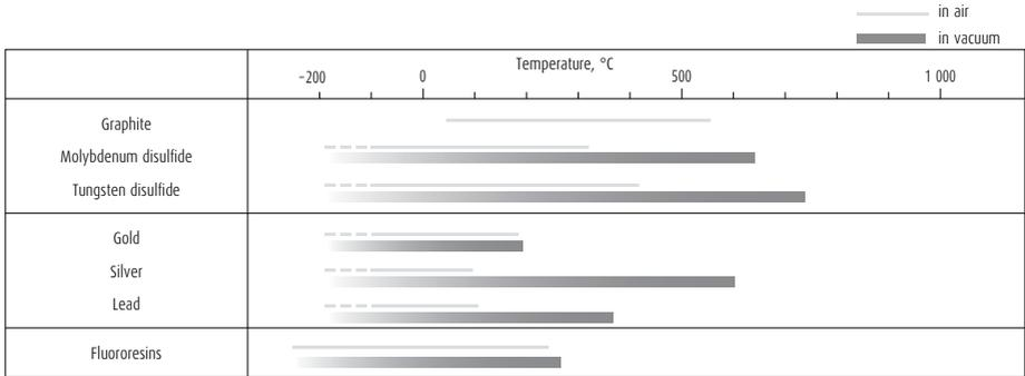
Fig. 2.7 Temperature range for using solid lubricants
