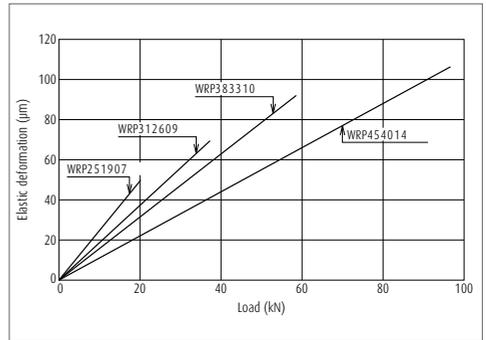
Fig. 4 Elastic deformation of the roller pack
