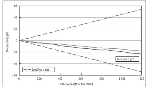
**Fig. 1** Example of measured variation in lead accuracy
