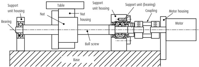
The screw shaft of the ball screw is supported by a nut and bearings, and it is driven by a motor.
