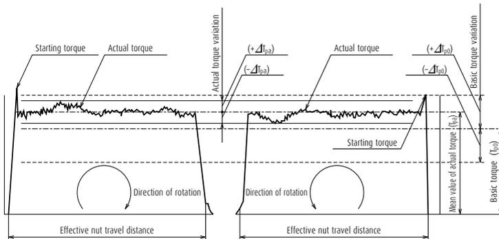
Fig. 7.2 Definitions of dynamic preloaded drag torque
