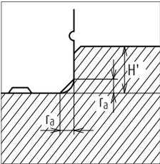
Fig. 5 Shoulder for the rail datum face
