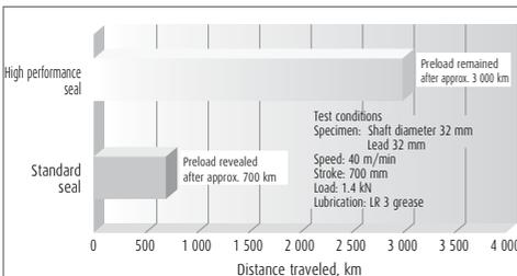
Fig. 3 Extreme durability test results using iron particles
