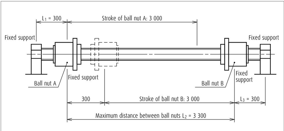
Fig. 8 Calculation example of permissible rotational speed
