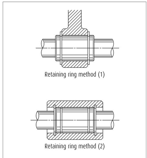
Fig. 9 Installation using retaining rings
