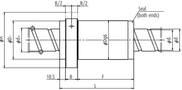
Screw shaft diameter  $d \geq 36$  mm
