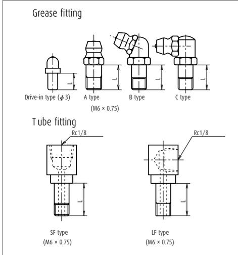
Fig. 1 Grease fitting and tube fitting
