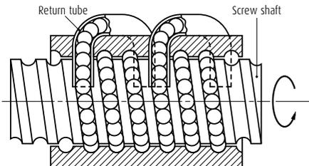
Fig. 1 Structure of return tube recirculation system
