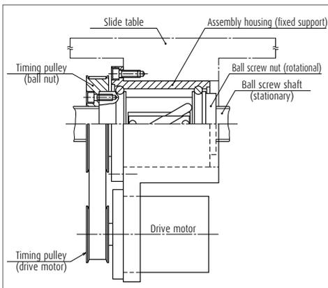
Fig. 2 Example of installation to the table
