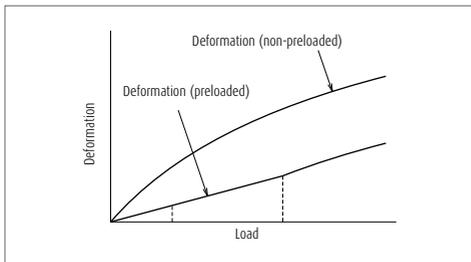
Fig. 3.9 Elastic deformation
