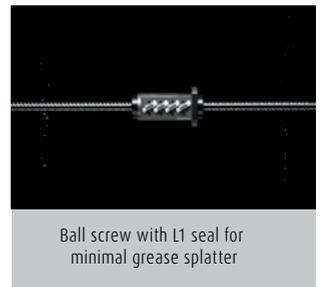
Fig. 2 Results of grease splattering test
