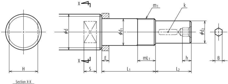
Fig. 4.6 R Series shaft end (drive side)
