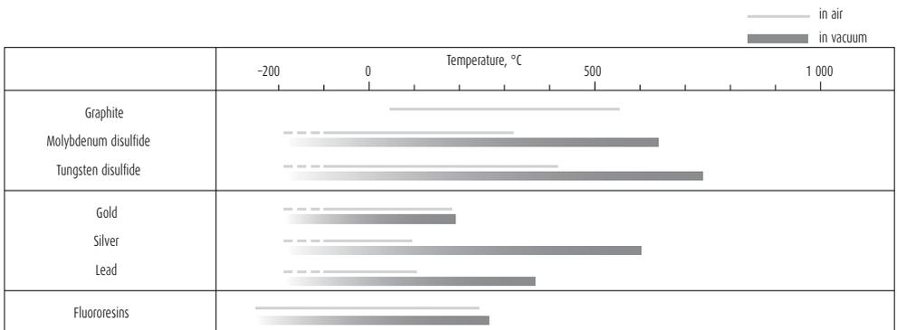
Fig. 9.8 Temperature range for using solid lubricants
