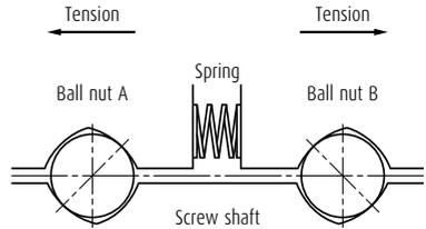
A spring is used as a spacer of D-Preload. Must be used with discretion in its varied rigidity by load direction.
