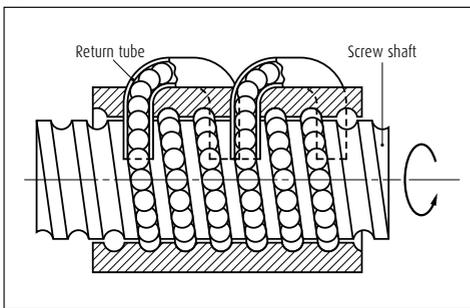
Fig. 1 Structure of return tube recirculation system
