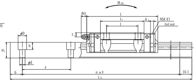
Specification for tapped holes on a rail bottom face
