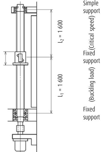
Fig. 16.7 Inspecting for buckling load and critical speed
