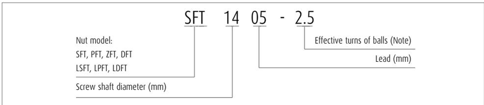
**Note:** In case of Z-preload, the number here is twice as large as the effective turns of balls.
