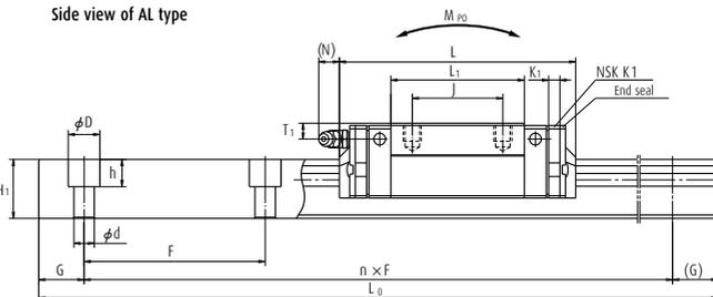
Specification for tapped holes on a rail bottom face
