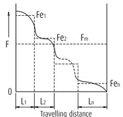
If the loads acting on the slider fluctuate (in general,  $M_p$  and  $M_y$  may fluctuate with the acceleration/deceleration of slider), the mean effective load is determined by Eq. 3).
