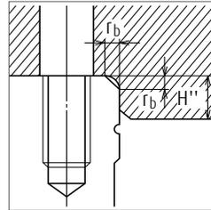
Fig. 10.11 Shoulder for the slide datum face
