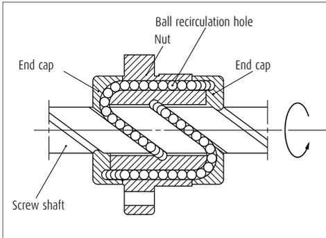
Fig. 1 Structure of end cap recirculation system
