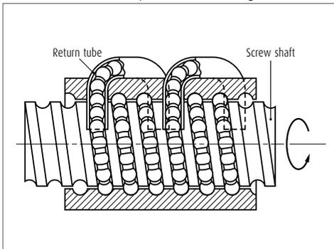
Fig. 1 Structure of return tube recirculation system
