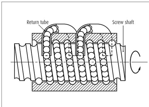
Fig. 3 Structure of return tube recirculation system
