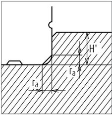
Fig. 9 Shoulder for the rail datum face
