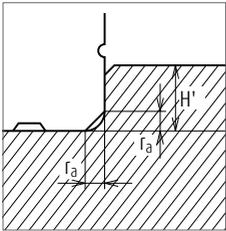
Fig. 9 Shoulder for the rail datum face
