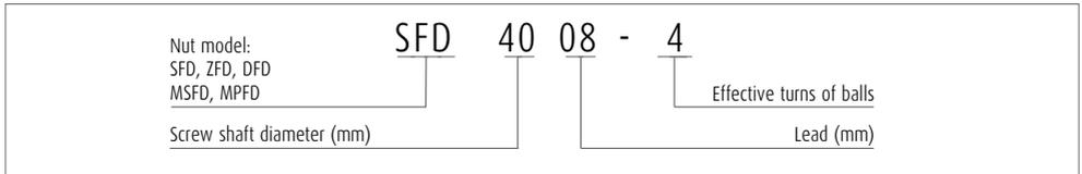
**Note:** In case of ZFD, the number here is twice as large as the effective turns of balls.
