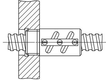
Fig. 15.6 Fixing a ball nut with thread screw
