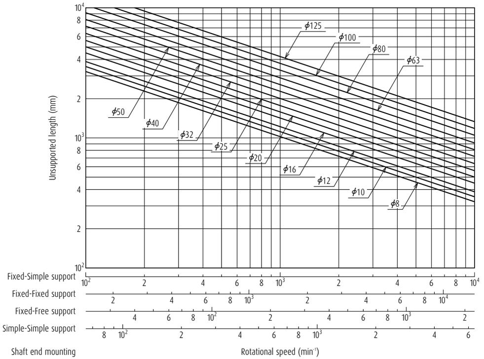
Fig. 3.1 Permissible rotational speeds vs. critical speeds
