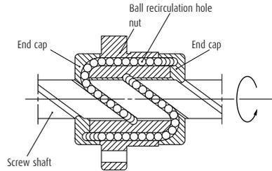
Fig. 3 Structure of end cap recirculation system
