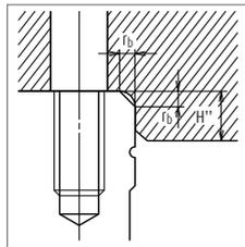
Fig. 11 Shoulder for the roller slide datum surface
