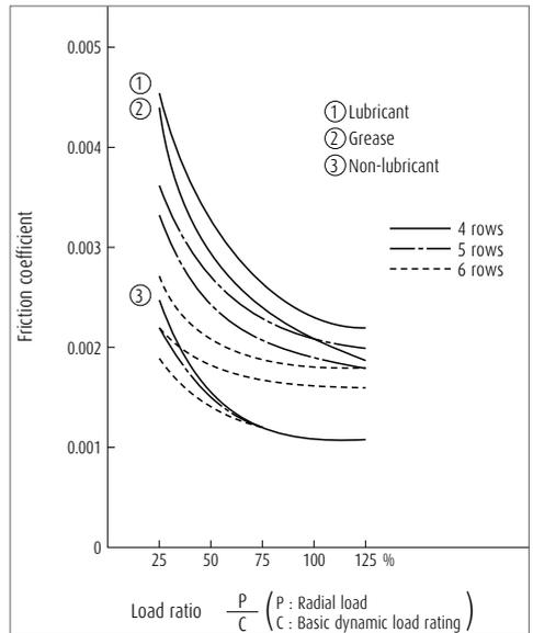
Fig. 4 Dynamic friction coefficient of linear rolling bushing
