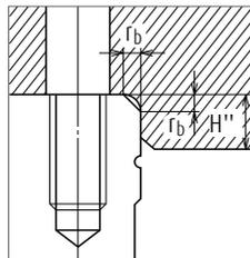
Fig. 6 Shoulder for the ball slide datum face
