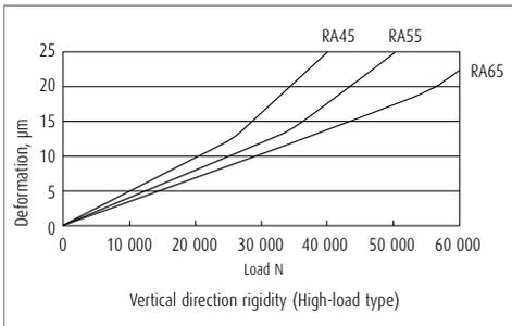
Fig. 6 Vertical direction theoretical rigidity line:
