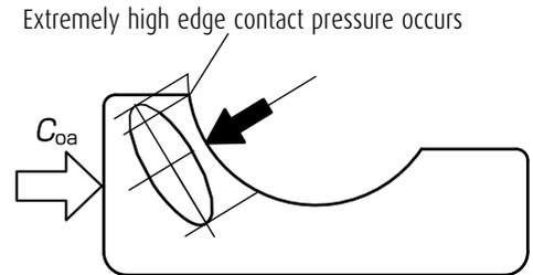
Fig. 6  $C_{0a}$  and limit axial load
