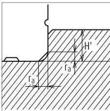
Fig. 8 Shoulder for the rail datum surface
