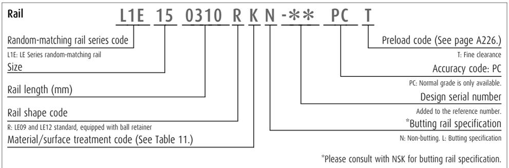
The reference number coding for the assembly of random-matching type is the same as that of the preloaded assembly. However, only the preload code of "Fine clearance T" is available (refer to page A226).
