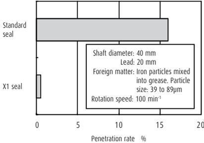
Fig. 1 Results of particle penetration rate test
