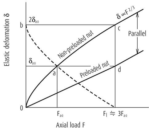
Fig. 6.3 Deformation of preloaded ball nut (position preload)
