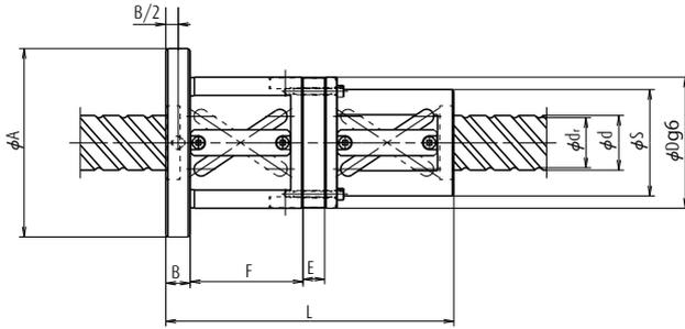
Nut model III (double nut spacer, preload)
