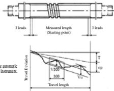
Laser beam type automatic lead measuring instrument.
