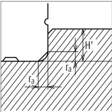
Fig. 9 Shoulder for the rail datum surface
