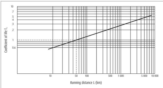
Fig. 5 Relationship between life factor and running distance
