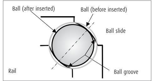
Fig. 3.1 Preloading method
