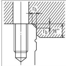
Fig. 7 Shoulder for the ball slide datum surface
