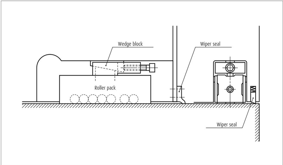
Fig. 6 Installation of seal
