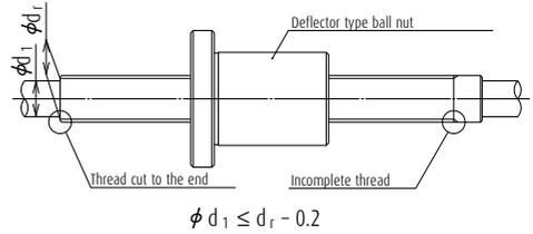
Fig. 15.1 Shaft end of a deflector recirculation system ball screw
