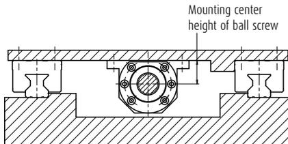
Fig. 4.2 Installation example
