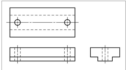
Fig. 2 Fitting plate
