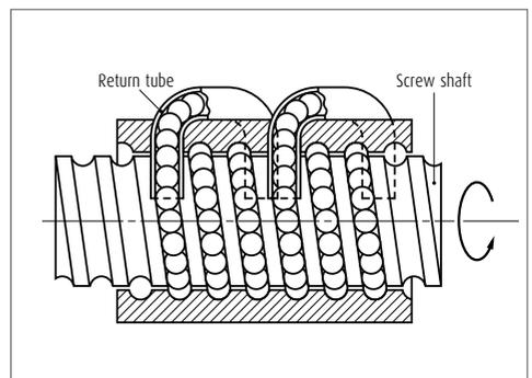
Fig. 3 Structure of ball return tube recirculation system
