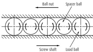
Balls slightly larger than the ball groove space (over-size balls) are inserted to allow them to contact at four points. Provides better torque characteristics in the low torque range.
