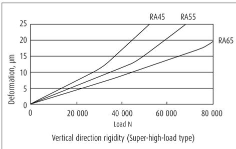
Fig. 7 Vertical direction theoretical rigidity line:
