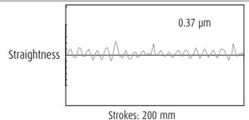
Fig. 6 Measurement results of HA Series and conventional Series
