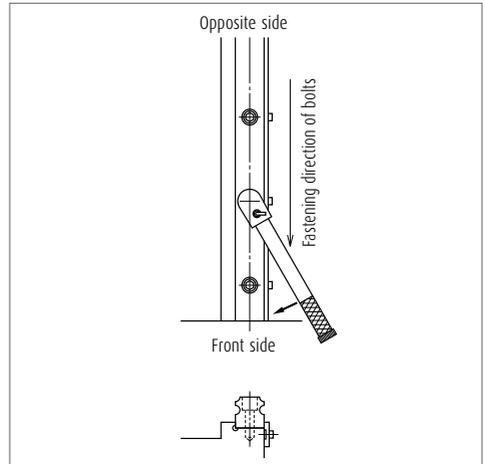
Fig. 10.14 Rail installation
