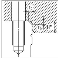
Fig. 6 Shoulder for the ball slide datum surface
