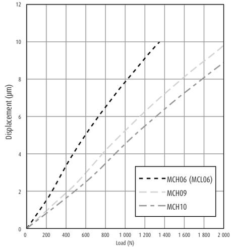
Fig. 4.3 MCH Series rigidity in radial direction
