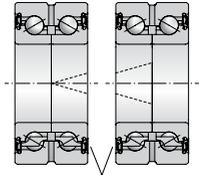
Distance between mating surfaces has been adjusted.
