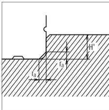
Fig. 10 Shoulder for the rail datum surface
