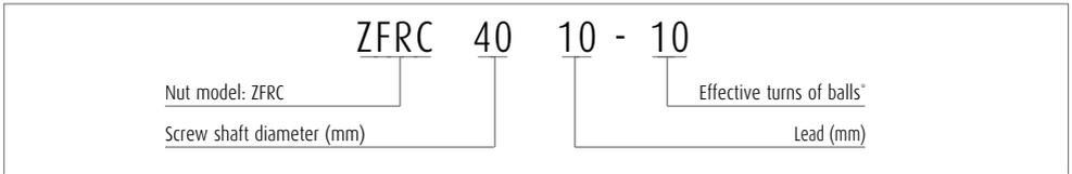
\* In the case of Z-preload, the amount shown is twice the effective turn of balls.
