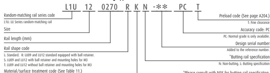
L: Standard. R: LU09 and LU12 standard equipped with ball retainer.
