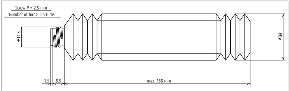
Fig. 1.1 Bellows tube
