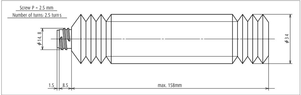
Fig. 6.6 Bellows tube
