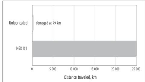
Fig. 6.2 Durability test at high speed, with no lubrication (lubricated by NSK K1 only)
