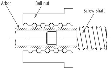
Fig. 15.4 Arbor to install and remove nut
