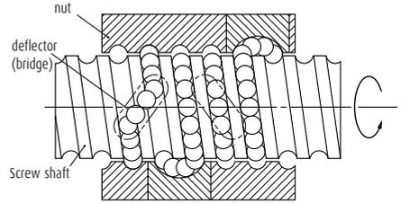
Fig. 2 Structure of deflector (bridge type) recirculation system
