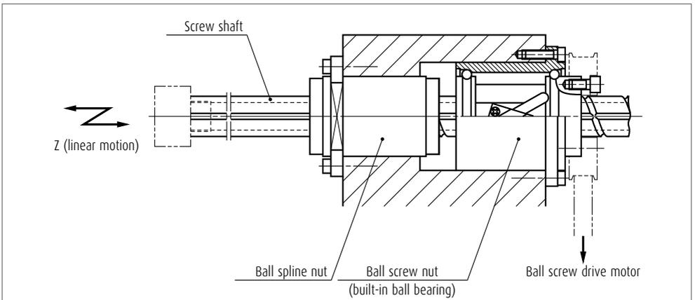
Fig. 2 Example structure of single Z axis unit
