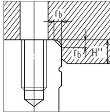
Fig. 6 Shoulder for the ball slide datum face
