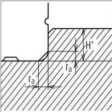
Fig. 5 Shoulder for the rail datum surface
