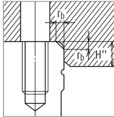
Fig. 10 Shoulder for the ball slide datum face
