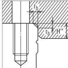
Fig. 10 Shoulder for the ball slide datum surface
