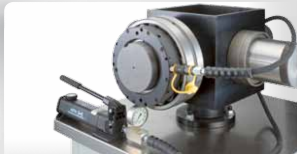
Extraction of the withdrawal sleeve with a hydraulic nut
