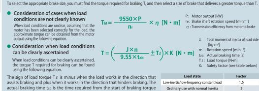
generation until braking is complete. When this is not clearly known at the selection stage, a guideline value is used that factors in service life and the like.
