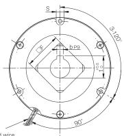
Lead wire length: 400 \*The lead wire extraction position for size 14° is 60°.
