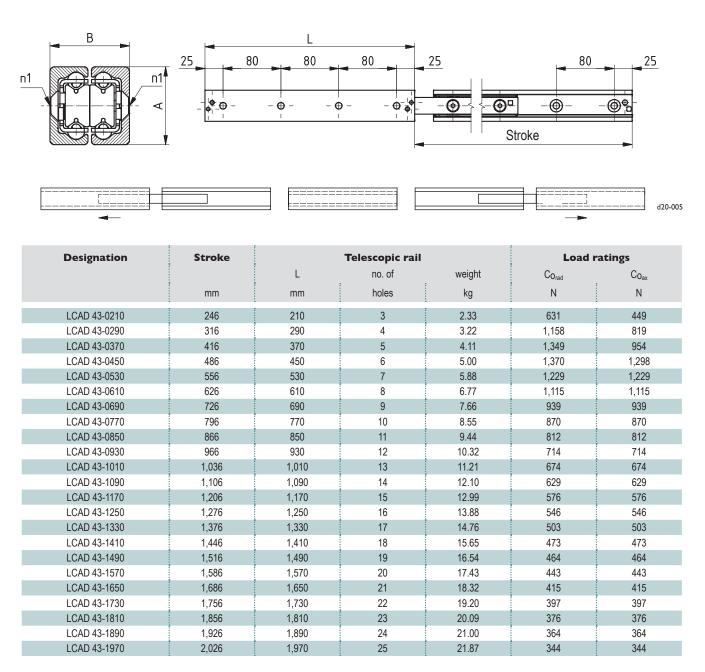
If the stop screws are removed, then the overall two-way stroke will be twice the stroke specified in this table.
