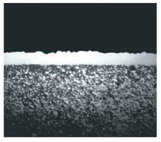
Fig. 8.2: Cross section of the ATCoat coating
