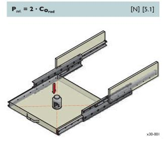
Fig. 5.1: Presumed point of load application for paired installation
