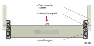
Fig. 6.1 Mounting recommendation for the LCAS and LCBS Telescopic-Runners
