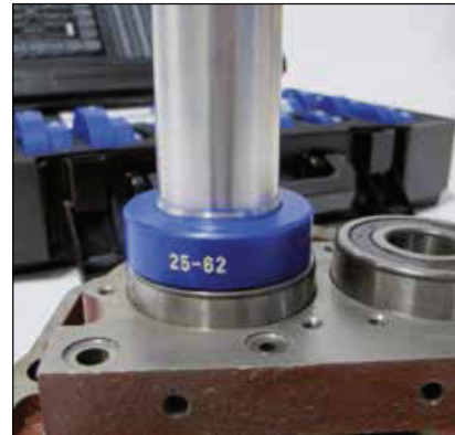
Collets are engraved and marked clearly
