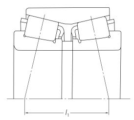
Fig. 5-1 Back-to-Back Arrangement
