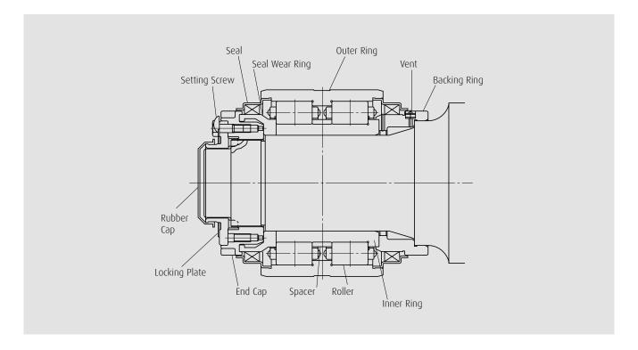
Fig. 3-1 Sealed-Clean Rotating End Cap Cylindrical Roller Bearings
