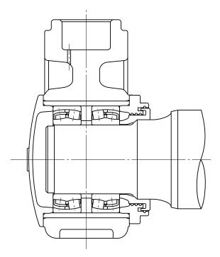
Spherical roller bearings can sustain, not only heavy radial loads, but also some axial loads in either direction. They have excellent radial load carrying capacity and are suitable for use where there are heavy or impact loads.
