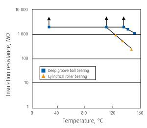
Fig. 7-3 Temperature vs. Insulation resistance
