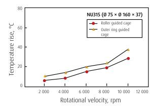
Fig. 7-2 Comparison of temperature rise
