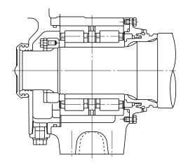
Double-Row Cylindrical Roller Bearing with Rib to Sustain Axial Load
