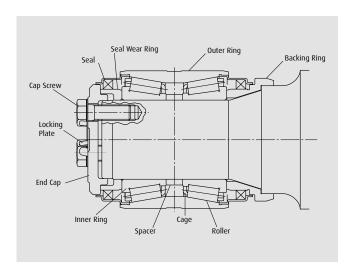
Fig. 2-2 Sealed-Clean Rotating End Cap Tapered Roller Bearings
